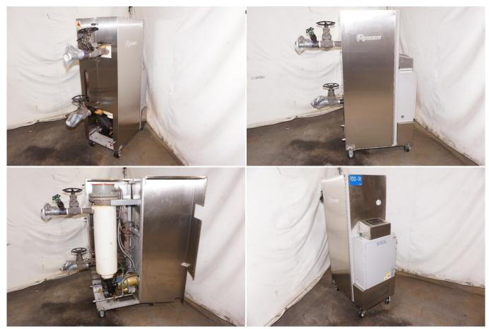
**Description:** Used, Advantage Model RK4-48100HC 48 kW Single Zone Portable Hot Oil Process Heater Temperature Control Unit with Cooling Water Circuit For Sale, Features include: Regal RK with G500 Series Controller, Water Cooling Circuit, Built-in pump pressure relief valve, Unit on casters for easy movement, , , Regal G500 Series Controls, Second Hand, DCM-5291
